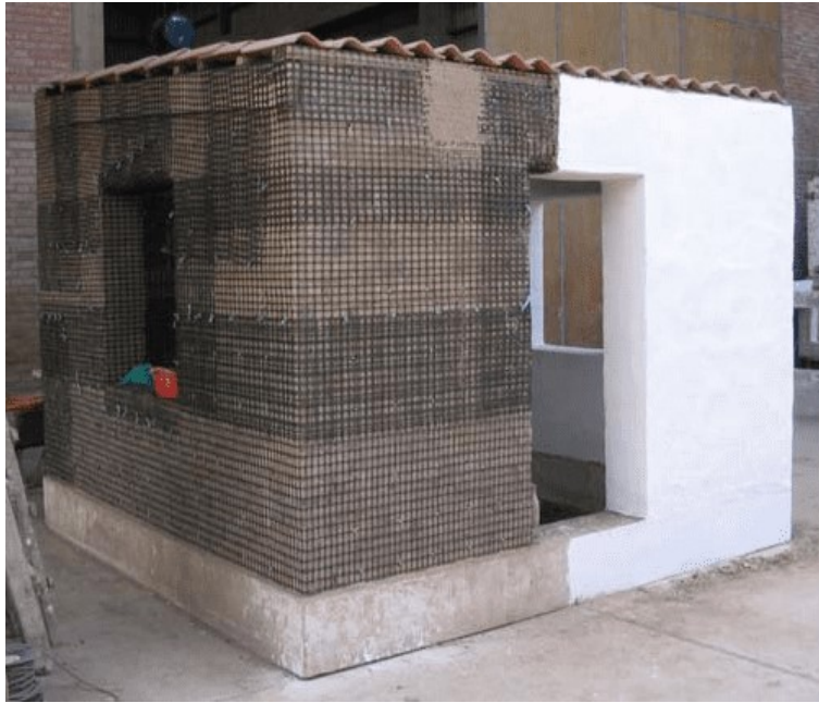
Adobe test-house reinforced with polymer mesh and partially plastered.
